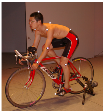
Fig. 12 Captured points in cycling motion. (White points on the human body represent markers for optical motion capturing system.)
